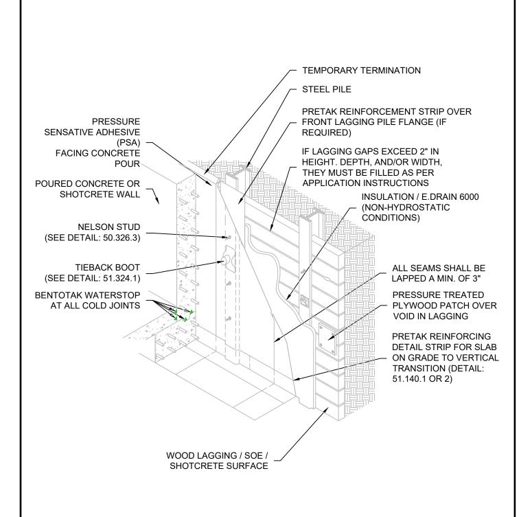
G:\My Drive\Epro Master Folder\Drafting\Details\Shoring\Pretak-HW\52.380.1 INSTALLATION OVER WOOD LAGGING AND STEEL PILES.dwg [Detail] November 20, 2020 - 2:35pm
