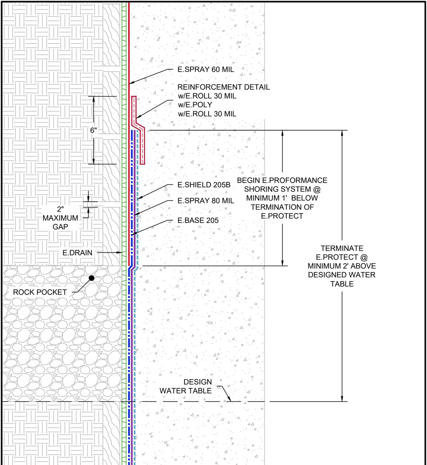
G:\My Drive\Epro Master Folder\Drafting\Details\Transitions\Hybrids\Shoring To Shoring\2.350.2.01 E.PROTECT SHORING ASSEMBLY TRANSITION TO E.PROFORMANCE SHORING ASSEMBLY w/ROCK POCKET.dwg [Detail] June 29, 2021 9:19am
