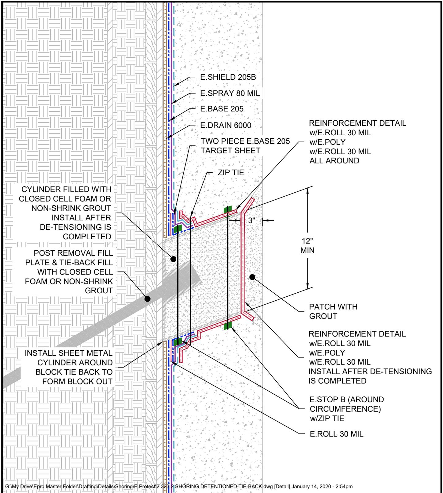
G:\My Drive\Epro Master Folder\Drafting\Details\Shoring\E.Protect2.323.2 SHORING DETENTIONED-TIE-BACK.dwg [Detail] January 14, 2020 - 2:54pm
