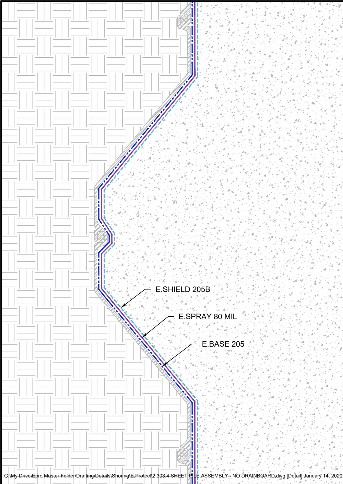
G:\My Drive\Epro Master Folder\Drafting\Details\Shoring\E.Protect\2.303.4 SHEET PILE ASSEMBLY - NO DRAINBOARD.dwg [Detail] January 14, 2020 - 11:47am
